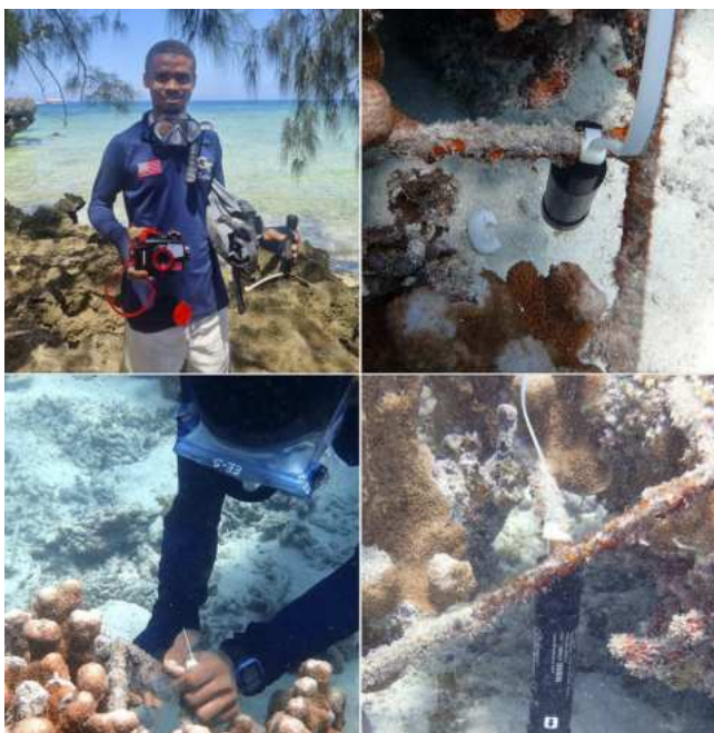
Figure 35. Installing HOBO monitoring equipment in the CRS.
